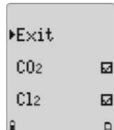
7. Attach the calibration cap and apply gas at a flow rate of 500 ml/min.
