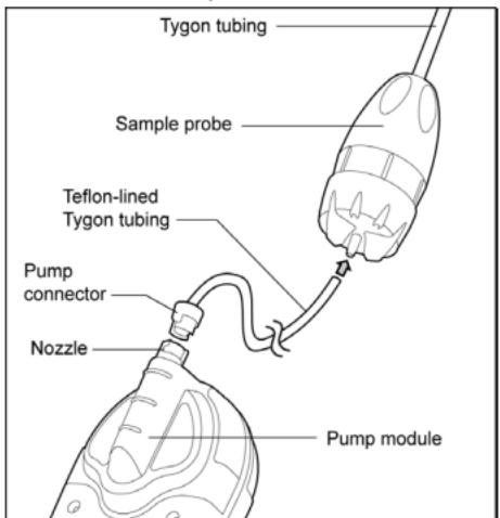
The detector and pump module can also be used with a sintered filter.
