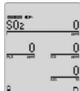
8. When the span is complete, the following three screens display:
