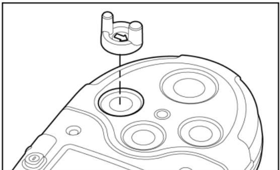
2. Connect the calibration hose to the gas cylinder and to the intake inlet on the cap.
