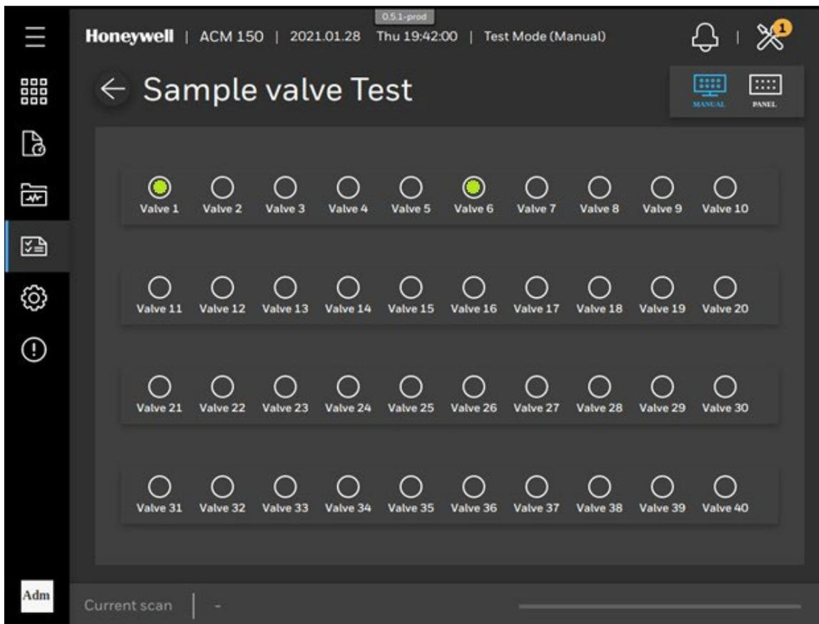
Figure 75. Sample Valves Manual Control
