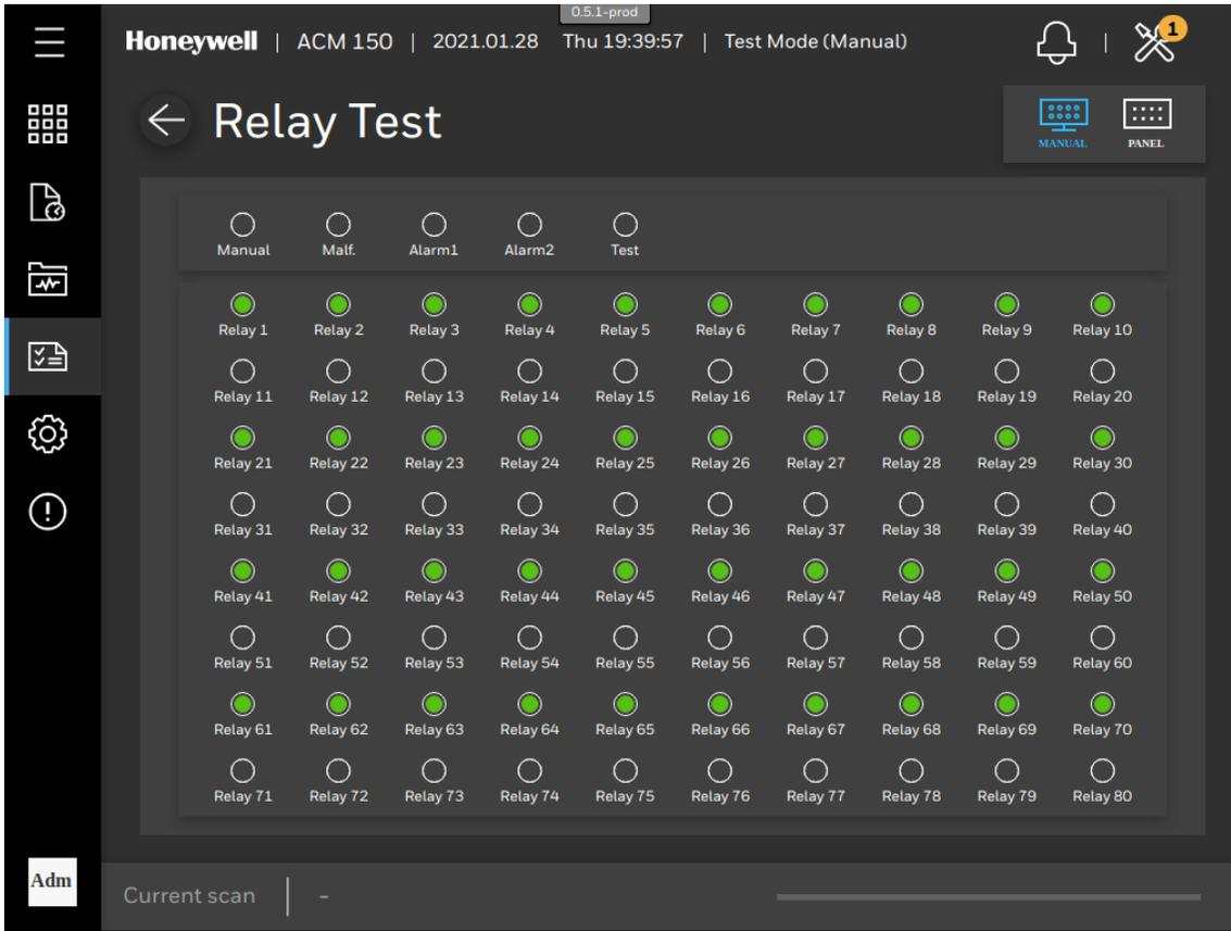
Figure 76. Relays Manual Control
