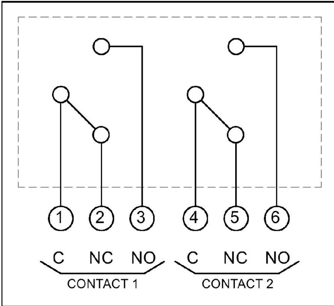
Figure 16. Relay Schematic
