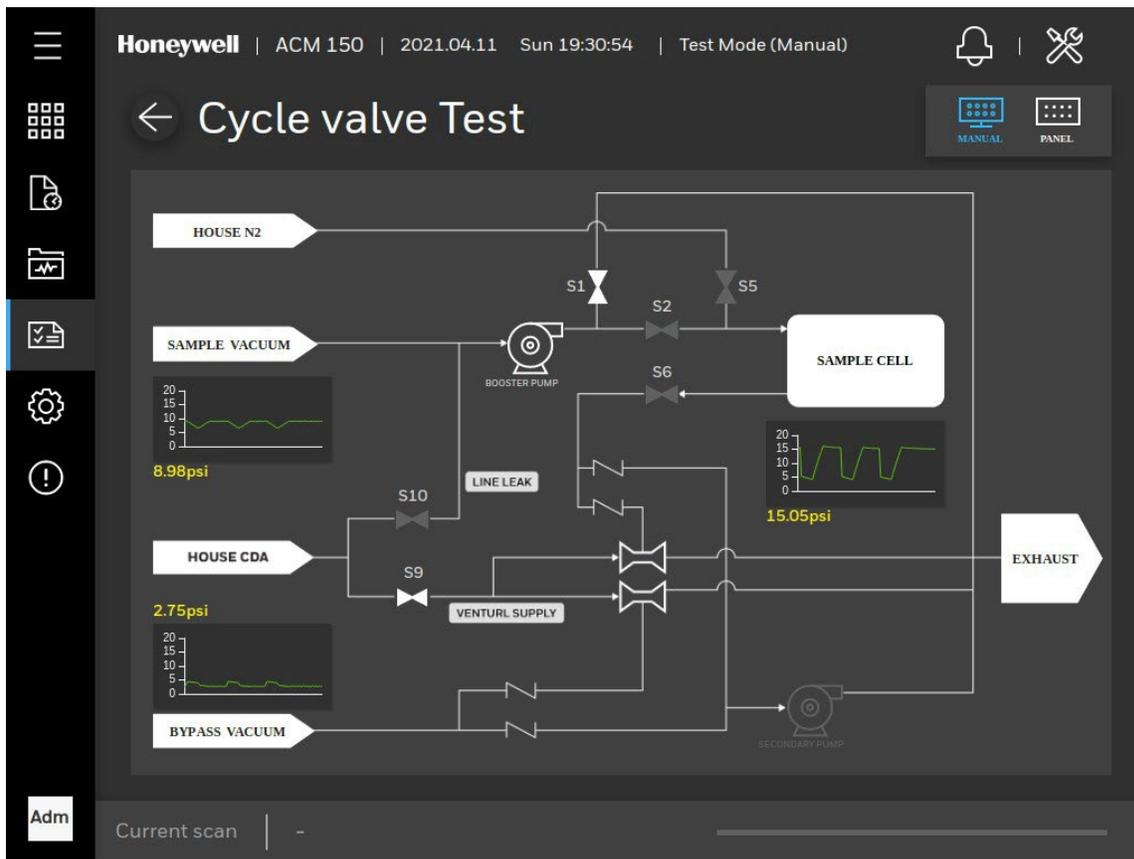
Figure 74. Cycle Valve Test (Venturi pump, line leak option)
