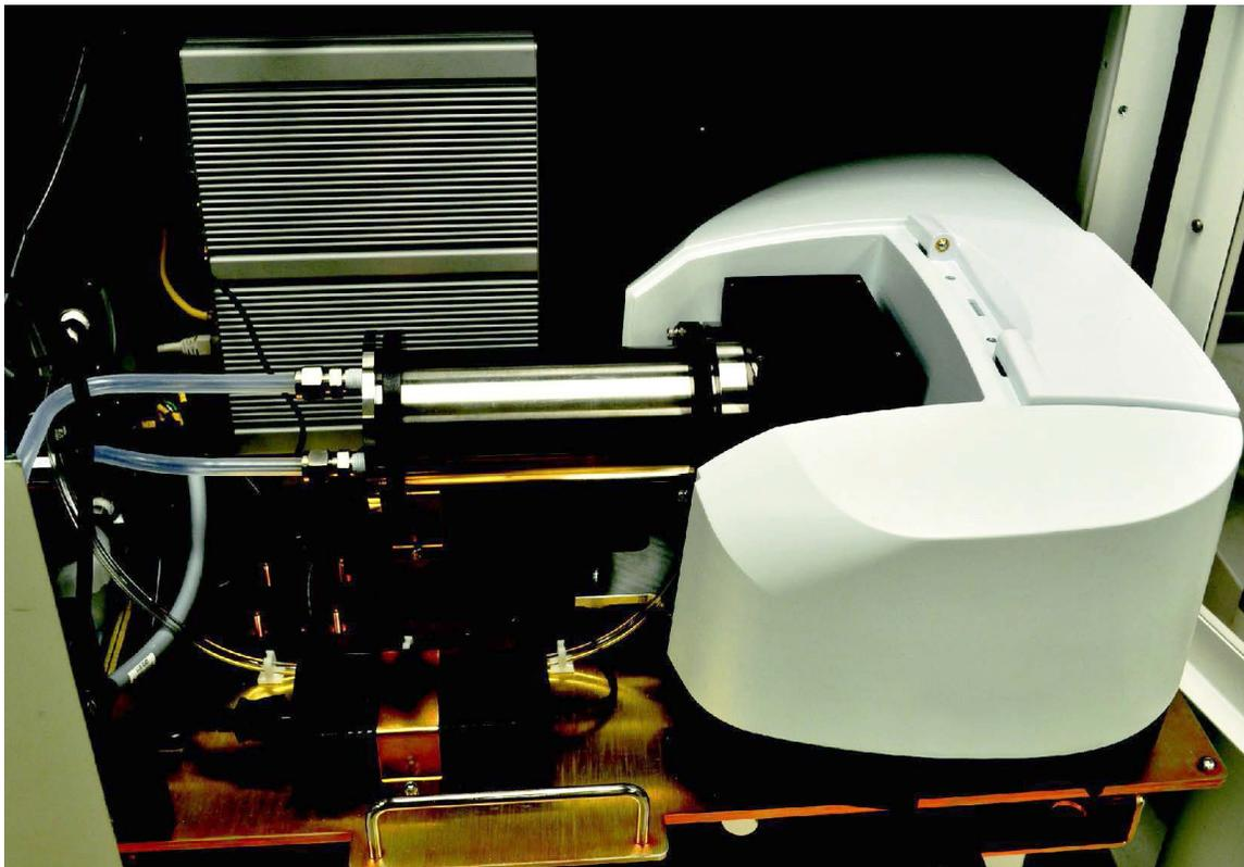
*Figure 13. FTIR Bench Assembly*
