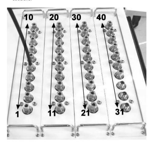
Figure 26. ACM 150 Tube connection points
