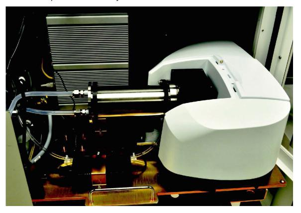
Figure 13. FTIR Bench Assembly
