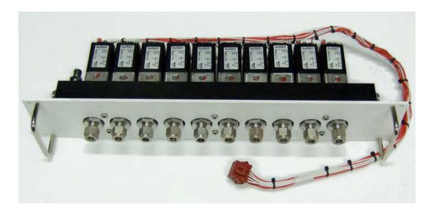
Figure 5. 10 Sample Valve Manifold
