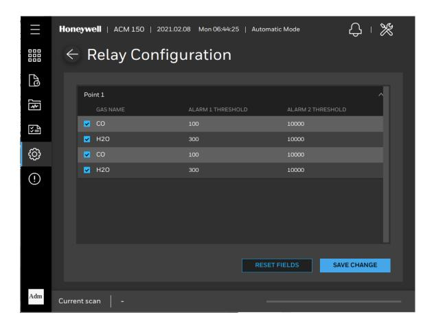
Figure 63. Selecting Relay Gases
