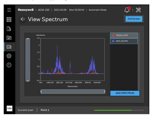
Figure 49. Spectrum Overlay
