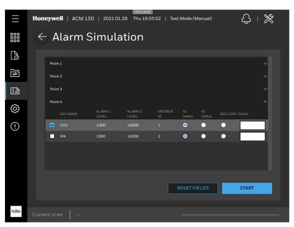
Figure 79. Alarm Simulation
