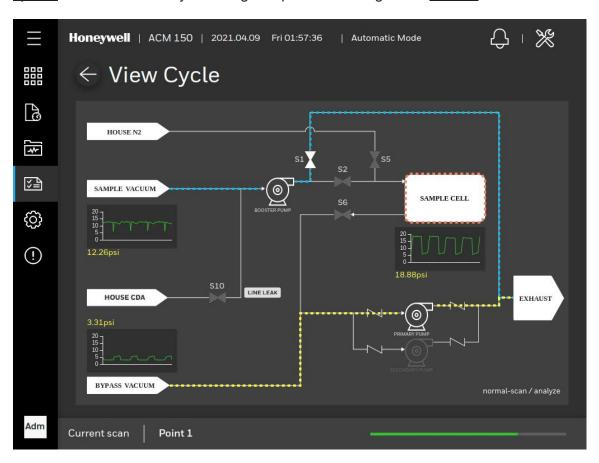
Figure 71. View Valve Cycles
