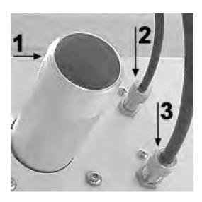
Figure 25. Nitrogen, CDA, and Exhaust Connections
