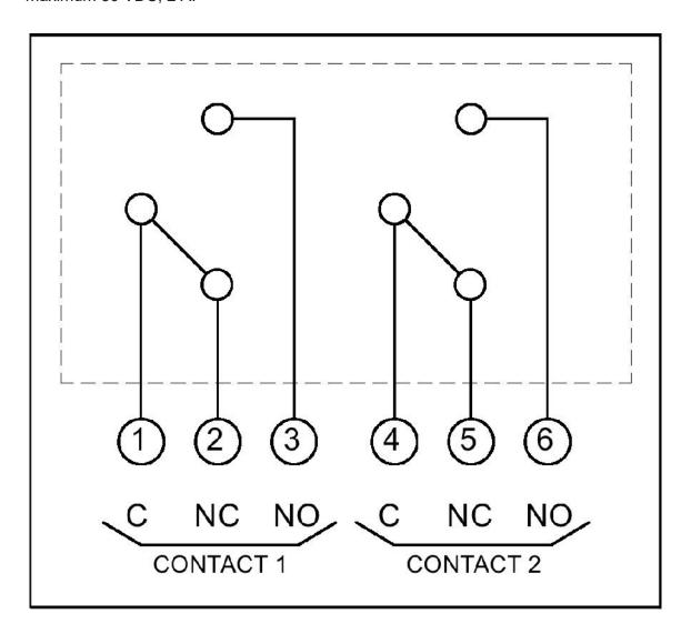
Figure 16. Relay Schematic
