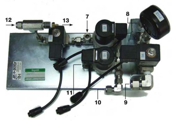
Figure 9. Cycle Valve Assembly
