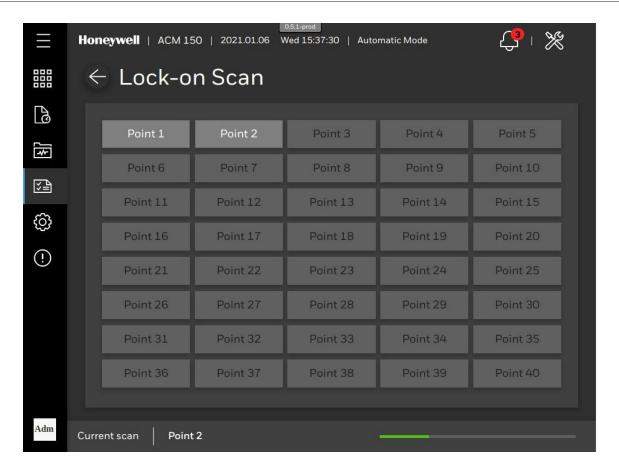
Figure 40. Select a Point Lock-on Scan
