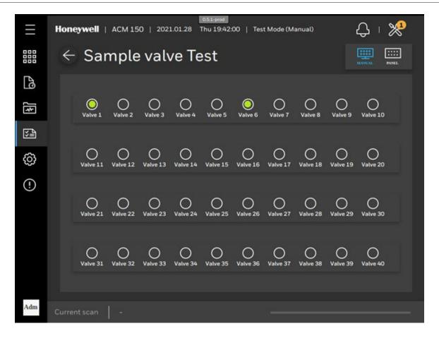
Figure 75. Sample Valves Manual Control
