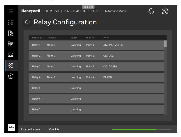
Figure 61. View Relay Configuration
