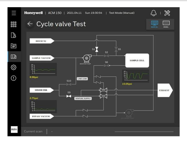
Figure 74. Cycle Valve Test (Venturi pump, line leak option)
