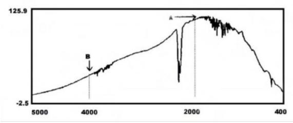
Figure 81. Correct Background Spectrum
