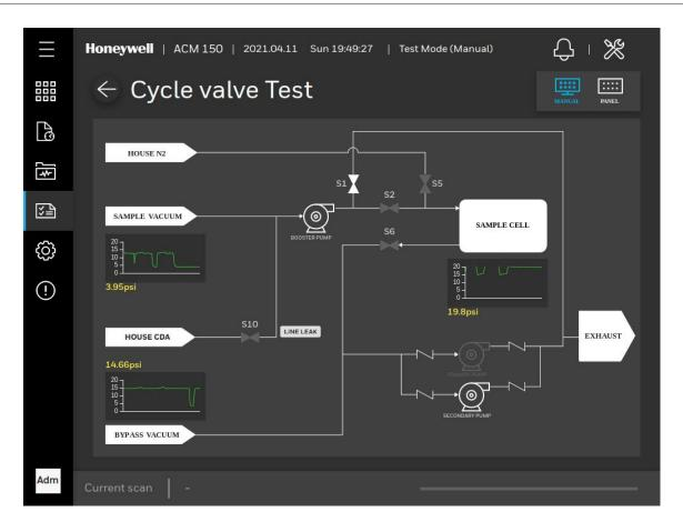
Figure 73. Cycle Valve Test (Dual pump, line leak option)
