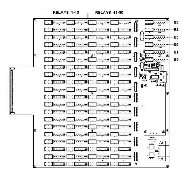
Figure 15. Relay Output Board
