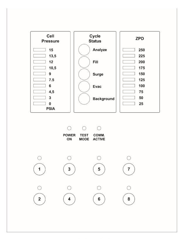
Figure 10. Cycle Valve Control Panel
