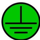
Figure 3. Protective Earth (Ground) Point
