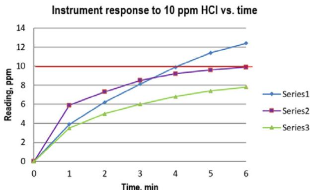
**Figure 1.** Results from three approaches to calibration for AreaRAE with HCl sensor.
