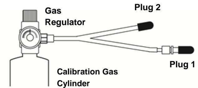
**Figure 2.** Fully assembled gas delivery system with cylinder, gas regulator and tubing.
