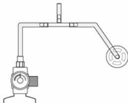
5. Attach the other end to the flow regulator of a calibration cylinder with 5 ppm NO<sub>2</sub> calibration gas (unless otherwise specified). The flow rate should not be less than 750cc/min ("T" type connection).
