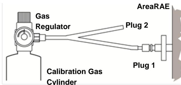
**Figure 3.** Attachment of gas delivery system to AreaRAE for calibration and bump testing.
