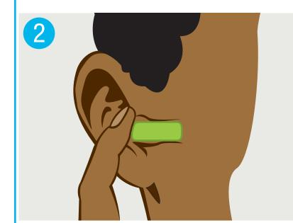
Earplugs should be inserted as shown in this drawing. Stop pushing earplug when your finger touches your ear.
