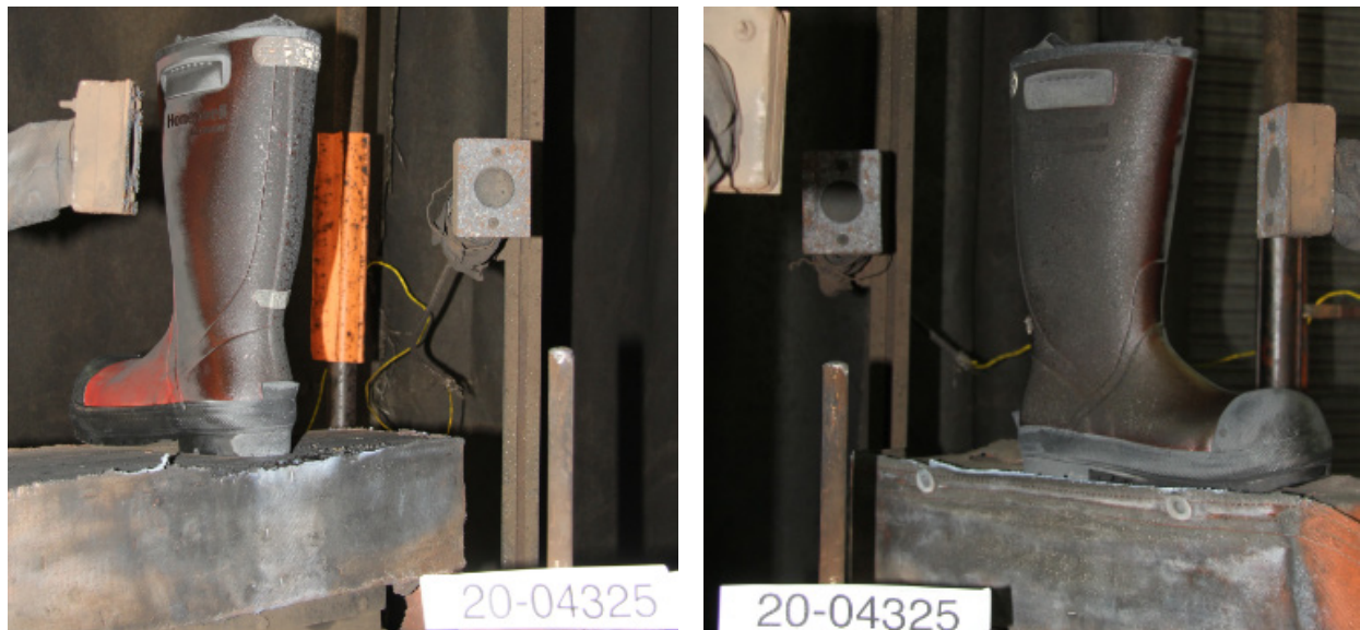
Figure 6.2: Boots as tested after arc exposure (left: A, right: B)..
