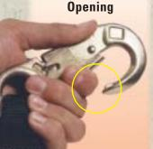
Shorter gate causes hands to interfere with throat opening, reducing clearance to 1/4" with hand and 1/8" with glove.
