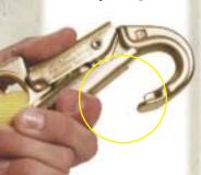
Longer gate permits lower hand position on a Miller snap hook, freeing the throat opening from obstructions. Clearance remains 3/4" with hand or glove for easy use.
