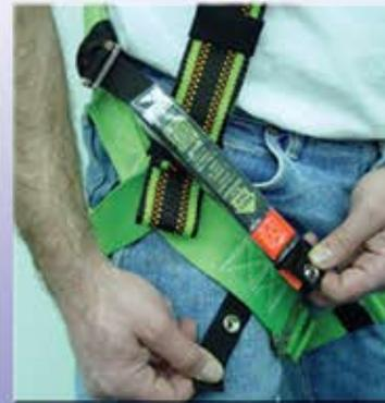
2. Attach "pull tab" button loop to the front leg strap above buckle.
