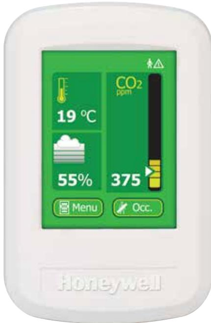
Improve indoor air quality and cut energy costs with CO<sub>2</sub> or VOC + temp/humidity monitoring for demand control ventilation. IAQPoint2 features a fully functional, multi-color, touch screen interface, the first of its kind. IAQPoint2 operates on +24 V<sub>AC</sub>/V<sub>DC</sub>. Analog output is 4-20 mA or 2-10 V<sub>DC</sub>, switch selectable. Digital output is BACnet/Modbus selectable or LonWorks. Available in wall mount and duct mount configurations.
