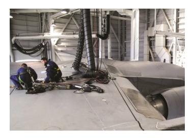
Aircraft maintenance requires workers to enter confined spaces that contain jet fuel vapors. As with all confined spaces, gas monitors are required to confidently decide if the atmosphere is safe for worker entry. Because of the physical qualities of jet fuel, specialized gas monitoring techniques should be considered.
