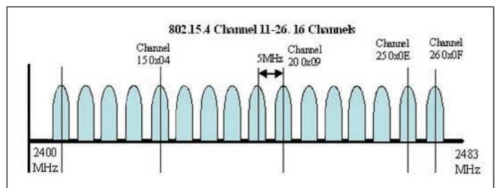
Figure 4. 802.15.4 frequency channels.
