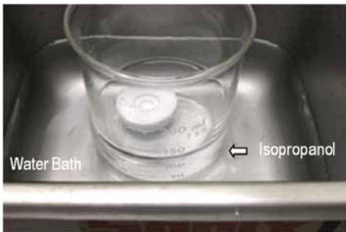
Figure 5. Sensor is cleaning in the ultrasound bath.
