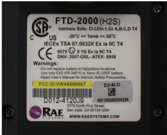
**Figure 2: MeshGuard Detector equipment certification label.**
