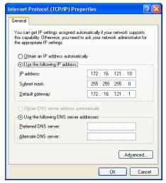
Figure 2. Manually Set PC network properties for connection to AutoRAE 2.
