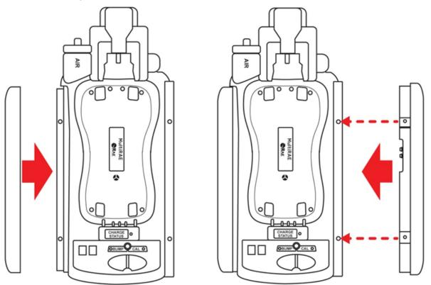
Slide the cap over the end and snap it into place.
