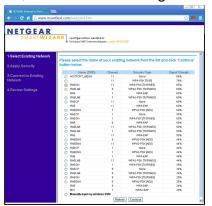
Figure 4. Select a wireless network. (This example shows all available wireless networks within range. Your choices will be different.)
