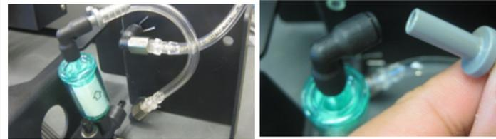
2. Using the flat screwdriver release the E-rings on the top and bottom of the flowmeter. (Recommend to use magnet to hold the E-ring when releasing.)
