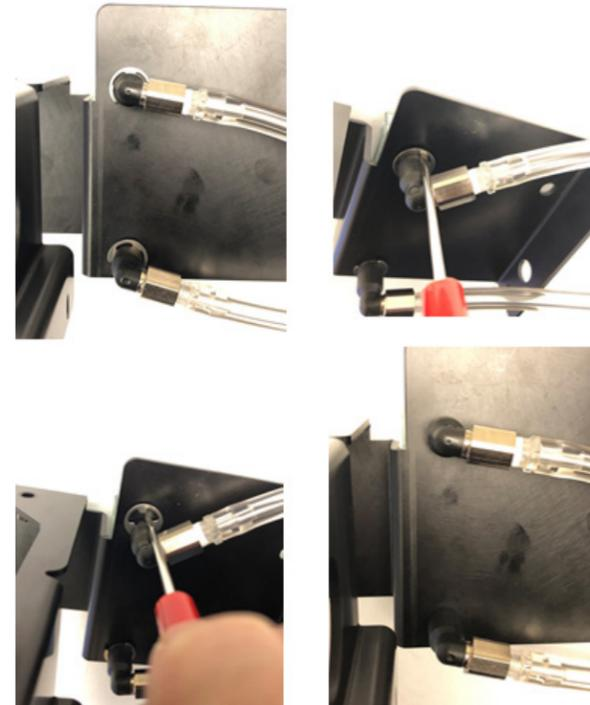
3. Pull the top and bottom of flowmeter to provide enough space for the flat screwdriver between the plate and fittings. Using the flat screwdriver release the fittings.
