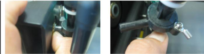
Install the new VI kit by first pushing the VI tube end into the manifold on the bottom. Ensure that the VI Kit is completely seated in the manifold. Push the other tube end into the SPM inlet and push until VI Kit cannot go in any farther. NOTE: The manifold must remain on the two threaded post at all times.
