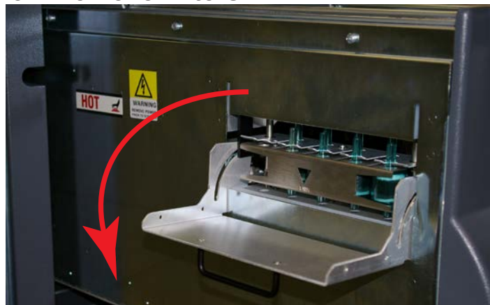
Figure 5-5. Pyrolyzer Filter Door
