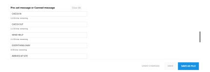
Note: Your messages are limited to 20 characters each, including spaces and hyphens. Text is automatically divided into lines at word spaces and hyphen characters. Therefore, you should include word spaces or hyphens. Otherwise, it cannot create a new line when necessary.
