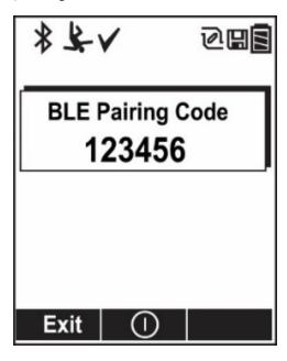
Type the pairing code into mobile app to pair the instrument and the smartphone/mobile app.
