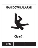
In addition, the instrument alarms (audible and visible) four times per second. The instrument also sends an emergency message to Safety Suite Device Configurator (SSDC).
