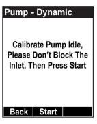
Press [MODE] to begin calibration. There is a countdown shown in the box. Press [N/-] anytime to abort the calibration.
