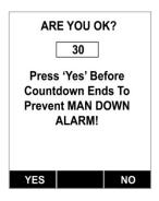
If you do not need assistance, press [Y/+] before the countdown reaches 0 to stop the Man Down alarm from being activated. Otherwise, press [N/+] to trigger the Man Down alarm immediately, or do not press either key (the countdown will reach 0 and the alarm will start). When the Man Down alarm occurs, this screen is displayed:
