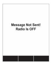
After a few seconds, the display automatically returns to the Send Message screen. Check that the radio module is turned on. If it is off, turn it on and try sending the message again.
