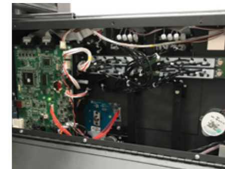
Step motor and encoder of Honeywell Vertex™ Edge
