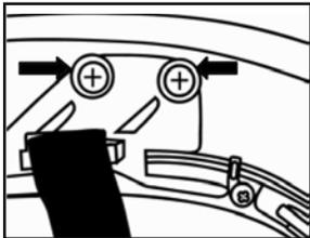
**Step 2 –** Unscrew the EZ Touch at each side of the suspension ring and remove the bushings.
