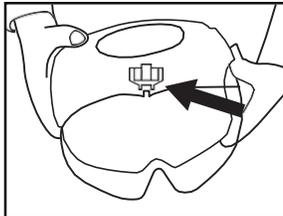
**Step 6 –** On the geared wheel mechanism side of the EZ Touch, align the two gears. Also align the hole in the EZ Touch with the hole in one-piece impact liner and suspension. Insert the bushing and screw, then screw them to the one-piece impact liner and suspension.
