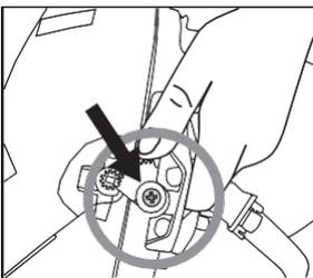
**Step 3 –** On the non-geared side of the one-piece impact liner and suspension, insert the post of the pre-loaded spring into the small hole
