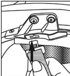
for a comfortable fit. To adjust, use the hex key provided. Turn the pictured small hex screw (on the left underside of the helmet brim) to
