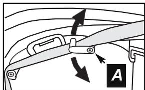
pull the goggle strap to the inside of the post. Rotate the post clockwise back to its original position forming a tunnel for the goggle strap.
