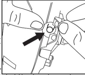
**Step 4 –** Insert the bushing and screw through the hole in the EZ Touch and screw them to the one-piece impact liner and suspension.
