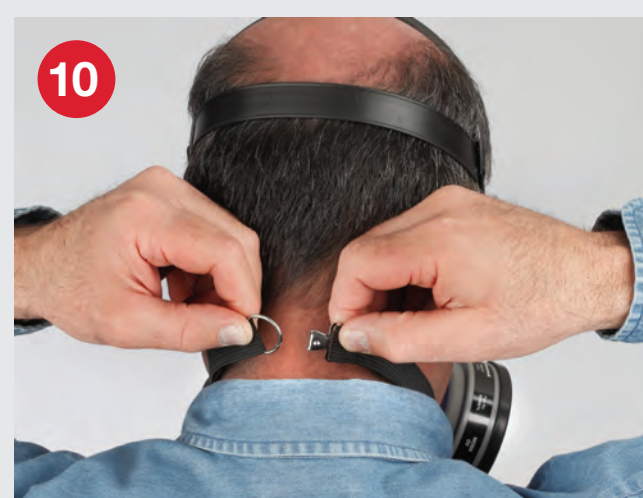
Fasten the bottom elastic straps behind your neck and under your hair. Remove any slack in the bottom straps by pulling the end tabs in the back towards the front. DO NOT TIGHTEN AT THIS TIME.
