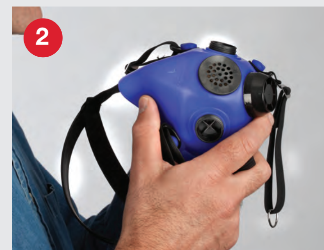
Check all the valves to be sure they are present and in good condition. They should be lying flat, without any distortion, tears or holes.
