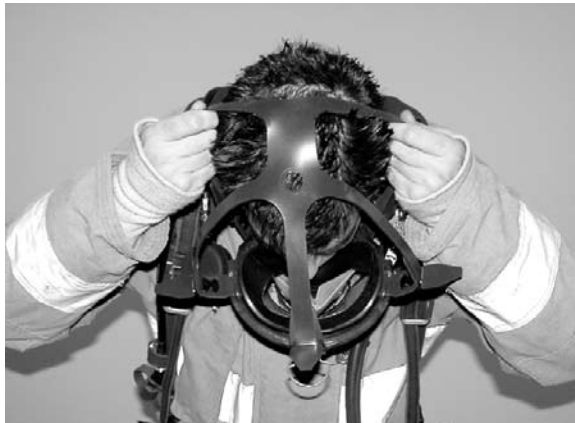
Figure 7. Grasp Lower Headstraps
