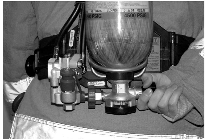
Figure 11. Open Cylinder Valve
