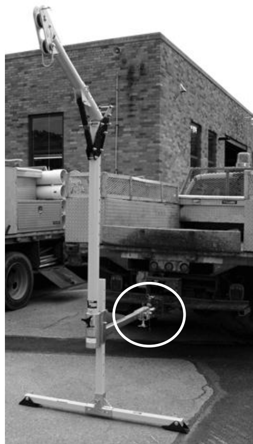
Pintle Hitch Adapter installed between the DH-12 and vehicle.
