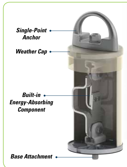
In the event of a fall, the Miller Fusion Roof Anchor Post orients in the direction of the force, the built-in, energy-absorbing component activates and the base remains securely attached to the roof surface.
