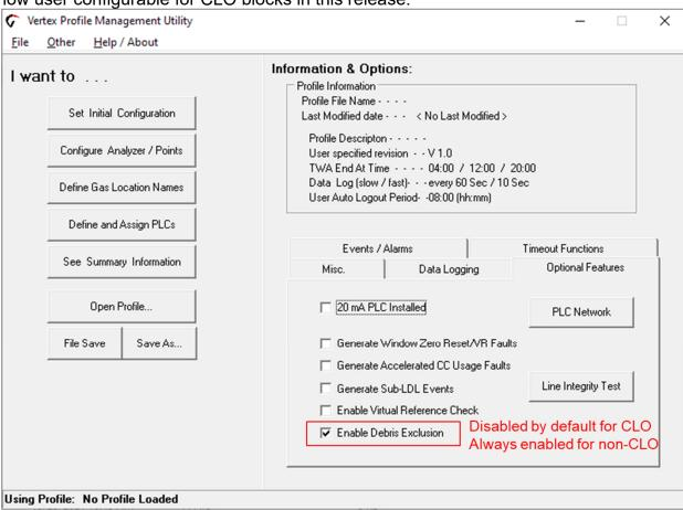
Enabling this feature may cause detection delay as high 10 seconds and extremely high concentration of gas may not be detected reliably.
