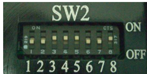
Eight (8) position DIP Switch (SW2) – Figure 3-2
