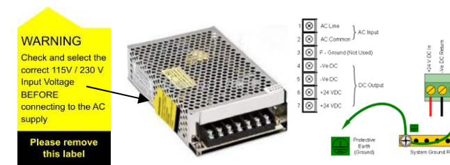
Figure 4. Switched Mode Power Supply (SMPS) Connections
