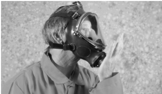
Figure 9. Fit Check for Conventional Facepiece
