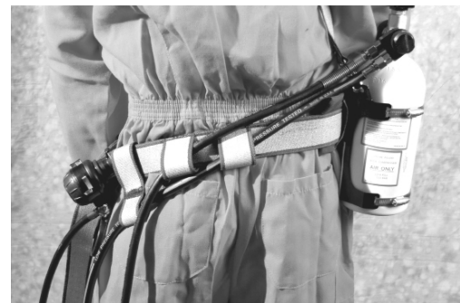
Figure 4. Routing of Hoses
