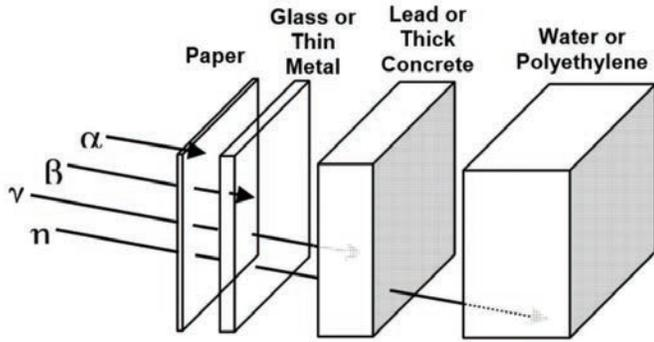
**Figure 2. Radiation Shielding.**
