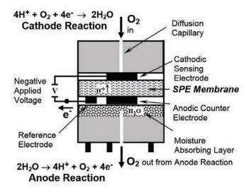
The amount of current necessary to reduce the incoming oxygen at the sensing electrode is proportional to the concentration of oxygen in the atmosphere being sampled. The net reaction of oxygen entering the top and leaving the bottom gives rise to the common name of "oxygen pump" for this type of sensor.
