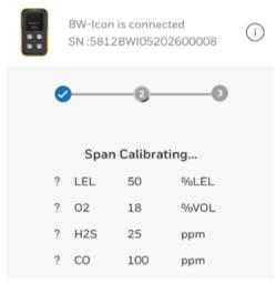
14. After calibration is complete, a report is displayed. Tap the Return Arrow button to exit the report and go back to the remote calibration main screen.
