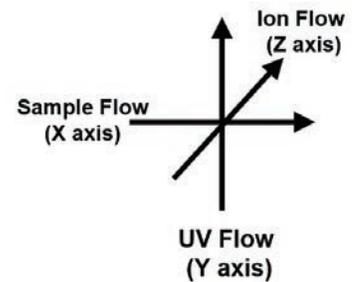
Rather they are fingers placed in the sample flow so that the ion flow is across the sample in the Z-axis. This sensor is used in the MiniRAE 2000, UltraRAE, and a variant of it is used in the ppbRAE.
