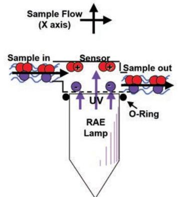
Together they form the second dimension. This sensor is used in the MiniRAE 2000, MultiRAE Plus, and ToxiRAE PID. The "2-D" sensor has a very small sensor chamber volume with a lower bias voltage and lower power requirements.
