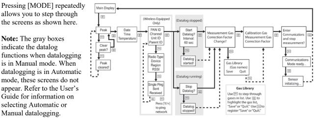
indicate the datalog functions when datalogging is in Manual mode. When datalogging is in Automatic mode, these screens do not appear. Refer to the User's Guide for information on selecting Automatic or Manual datalogging.
