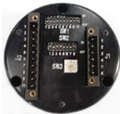
Figure 16. Electronics module, rear view (contacts shown with no power applied)
