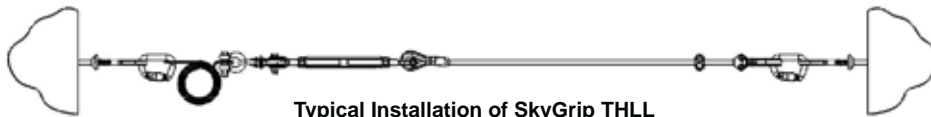
Typical Installation of SkyGrip THLL Using Model 494 Miller Mining Bolt Anchors or Model 497 Miller Grip Anchorage Connectors
