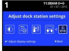
1. Press and hold **X** on the keypad until **Adjust dock station settings** is displayed on the LCD.
