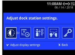
2. Press **◀** or **▶** on the keypad to select a settings option, and then press **✓** to display the option menu.
