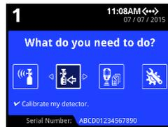
Calibration is a two-step procedure that determines the measurement scale for the detector's response to gas. In the first step, a baseline reading is taken in a clean, uncontaminated environment. In the second step, the sensors are exposed to known concentrations of gas. The detector uses the baseline and known gas concentrations to determine the measurement scale.
