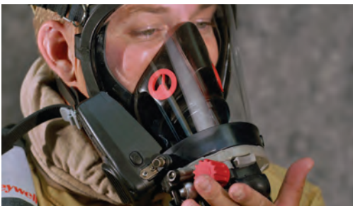
Figure 21. Insert the Regulator into the AIR KLIC
