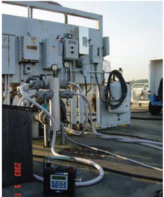
Figure 4. AreaRAE monitoring mechanical equipment.
