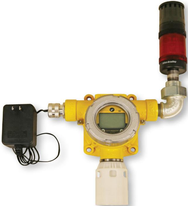
The Safe Area XCD with integrated horn and strobe allows the addition of audio and visual alarm indications to the XCD transmitter that incorporates relay outputs with 3/4" NPT threaded input ports. The Safe Area XCD includes the horn and light stack, 90° elbow, threaded nipple, strain relief, thread reducer, and a 0.67A 24VDC wall power supply. A stand alone solution for uncertified and general purpose areas.
