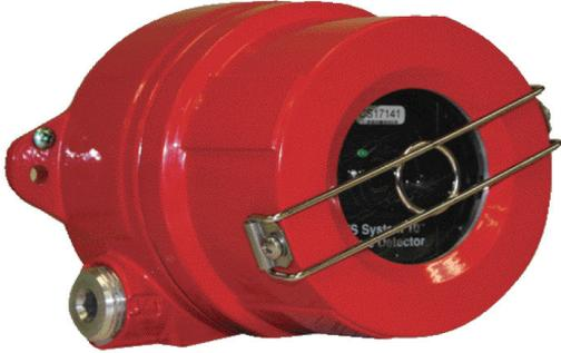
A high-speed microprocessor based fire detection and process control system specially designed for liquid and powder coating applications, the FS System 10 quickly detects the presence of a flame, reacts by initiating a shutdown of the electrostatic finishing process in a matter of milliseconds; and effectively interrupts the fire before residues and wet paint films can ignite.
