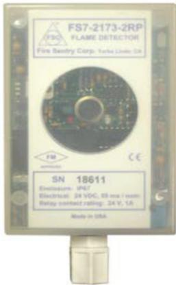
The Fire Sentry FS7 Flame Detector provides an intelligent two-stage response to semiconductor wet bench fires:
