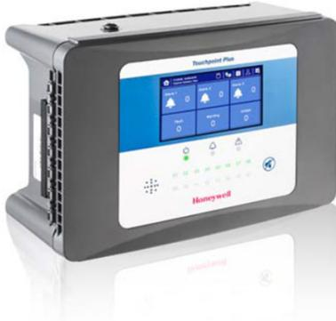
Touchpoint Plus is an easily configurable, wall mounted control system that supports up to eight channels of gas detection with a further eight channels available through an optional expansion unit. It accepts inputs from 2 or 3-wire mA or mV field devices.
