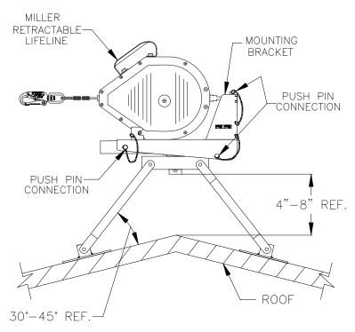
SHOWN MOUNTED ON A WOOD STRUCTURE WITH A MILLER MIGHTY LITE RETRACTABLE LIFELINE
