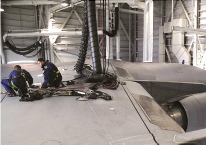
Aircraft maintenance requires workers to enter confined spaces that contain jet fuel vapors. As with all confined spaces, gas monitors are required to confidently decide if the atmosphere is safe for worker entry. Because of the physical qualities of jet fuel, specialized gas monitoring techniques should be considered.
