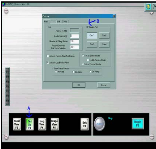
Figure 2. Set Up>>RF Modem Port. Press F2 (A) to activate “Set Up” dialog box, and proceed to select communication port that the RAE Link2 series modem is plugged into (B).
