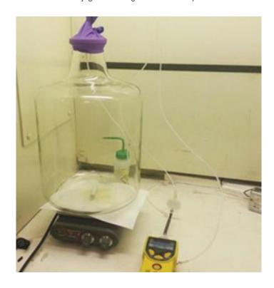
For a ToxiRAE Pro, use the plastic cap from the kit. Attach the cap with tubing to an additional external pump with a power supply to deliver gas from a jug to an instrument.
