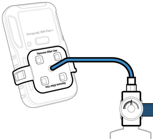
6. Apply span gas when the sensor slot LEDs start flashing. The bump test starts after the BW Flex Series detects gas. The four slots LEDs flash blue clockwise. After the bump test is completed, the LEDs are solid green if calibration passed, or red if failed.
