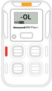
A Honeywell BW Flex-i handheld device with a monochrome screen displaying '-OL'. The device has a keypad and a speaker.          | "-OL" message is displayed. Intelliflash LED flashes amber. Alarmed sensor LED turns solid red.                   |
