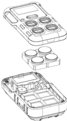
3. Put the new sensor in the correct sensor slot and notice the sensor's unfilled corner face to the sensor frame's unfilled corner. LEL and NDIR sensors are only supported in slot 1, and other sensors can work in any slot.
