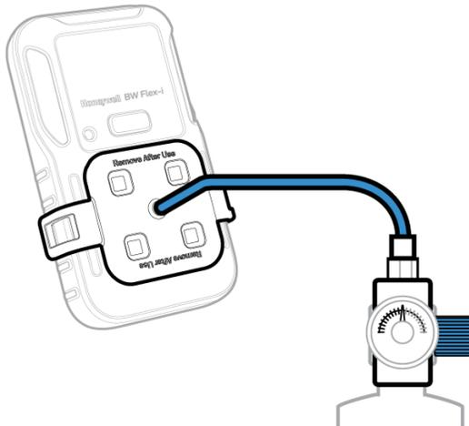
9. Apply span gas when the sensor slot LEDs start flashing. The bump test starts after the BW Flex Series detects gas. The four sensor slots LEDs flash blue clockwise. After the bump test is completed, the LEDs are solid green if bump passed, or red if failed.
