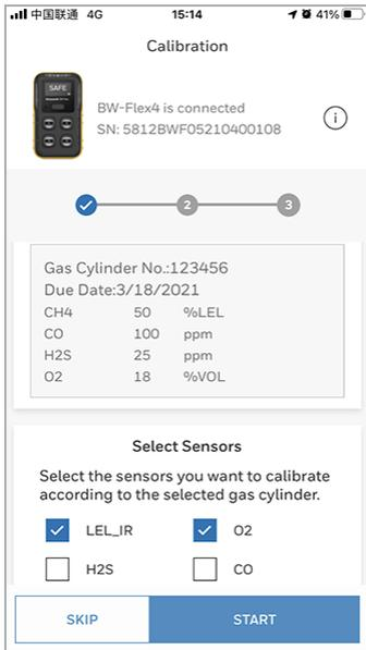
13. Open the cylinder valve by turning the pressure regulator knob counterclockwise. Follow onscreen instructions to know when to apply gas. The IntelliFlash lights amber.
