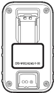
The model number should look like "CPD-W6X1H1M1-Y-00," the type of combustible sensor is identified by the 4th and 5th characters; in this case, "W6".
