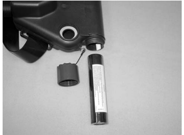
Figure 3. Rechargeable NiMH Battery Pack Installation
