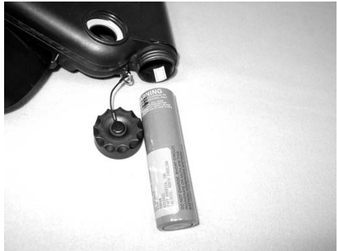
Figure 2. Non-rechargeable Li-SO 2 Battery Pack Installation
