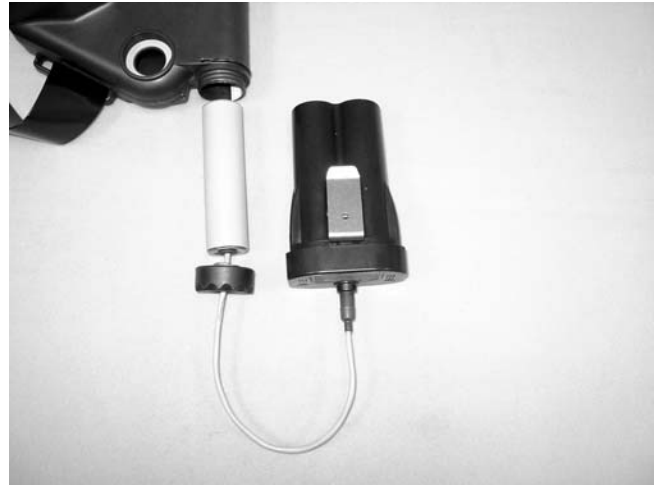
Figure 5. Alkaline Battery Pack Installation
