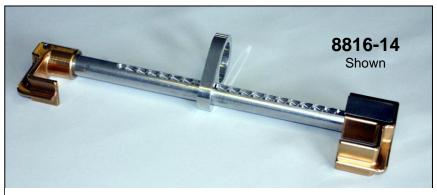
The Miller 8816-14 ShadowLite Beam Anchor connects to flanged beams ranging from 3 inches to 14 inches wide and up to 1-1/4 inches thick. Once locked on to the beam, the anchor grips the beam securely, yet moves freely with the worker along the beam to promote safety.
