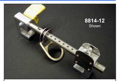
The Miller 8814-12 Shadow Beam Anchor is designed for use on I- and W-beams with flange widths ranging from 4 inches (100mm) to 12 inches (305mm) and flange thickness up to 1 ¼ inch. Once attached, the anchor will slide along the beam with the movement of the worker.
