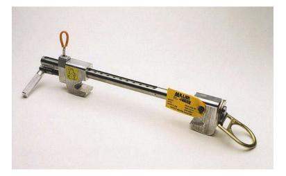
Miller Shadow Beam Anchors connect horizontally to a wide range of I and H beam flanges from 4 inches (100mm) to 24 inches (610mm) wide and up to 2-1/2 inches thick. The fixed unit (Model 8815) is designed to be tightened horizontally or vertically, firmly gripping the beam or column to provide a temporary or permanent anchorage attachment.
