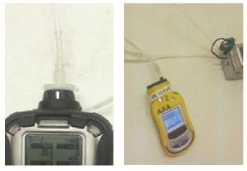
Connecting MultiRAE Pro and ToxiRAE Pro PID to the jug tubing.
