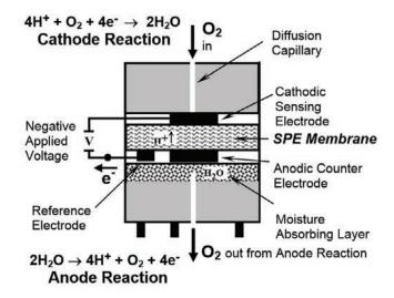
The amount of current necessary to reduce the incoming oxygen at the sensing electrode is proportional to the concentration of oxygen in the atmosphere being sampled. The net reaction of oxygen entering the top and leaving the bottom gives rise to the common name of "oxygen pump" for this type of sensor.
